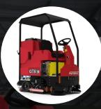
Overhead Guard protects operator from falling debris
