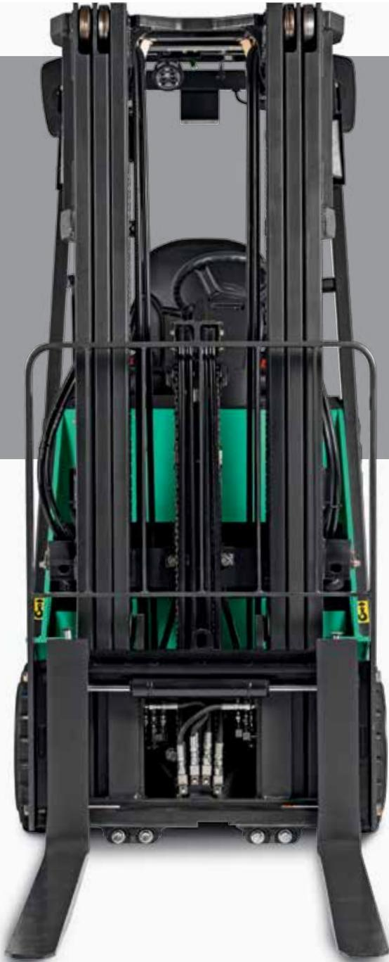
**Rock-Solid Frame:** The all welded box frame and battery edge cover design helps to extend the life of your investment.
