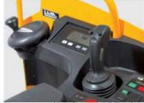
the operator with enhanced visibility. An All drive and lift functions are controlled by the multifunction joystick.
