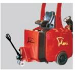
Low rear lift off or roll off for fast changeovers. Good access for battery topping. No electric motors, brakes or pumps underneath.
