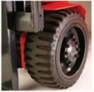
Flexi AC 1000 front twin drive wheels provide excellent grip and traction in slippery conditions when fully loaded. Continental MC20 super-elastic finger tread tyres for extended service life and resistant to damage.
