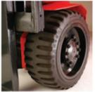
Flexi AC 1200 front twin drive wheels provide excellent grip and traction in slippery conditions when fully loaded. Continental MC20 super-elastic finger tread tyres for extended service life and resistant to damage.
