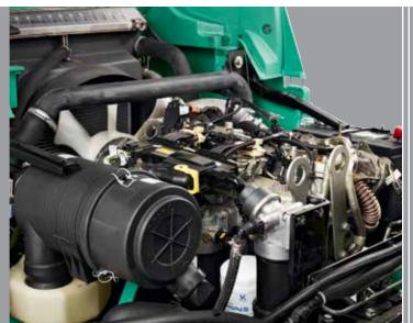
**Engine Protection:** Regulated by the Vehicle Control Module, the Engine Protection System keeps the truck running at desirable levels while helping to prevent damage to the forklift, saving you money. If the vital fluids become critically low, RPM levels are automatically lowered and the operator is immediately notified by a light on the dash display.
